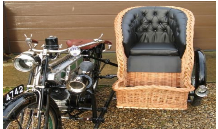
A sidecar for a Phelan & Moore 1912 motorbike
